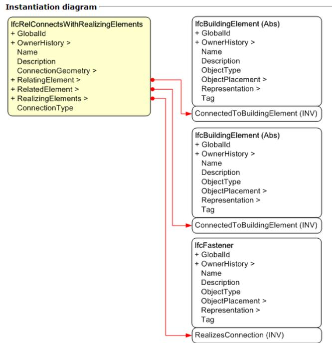
Figure 2: PCI-147: Instantiation diagram for precast joint element assignment.
