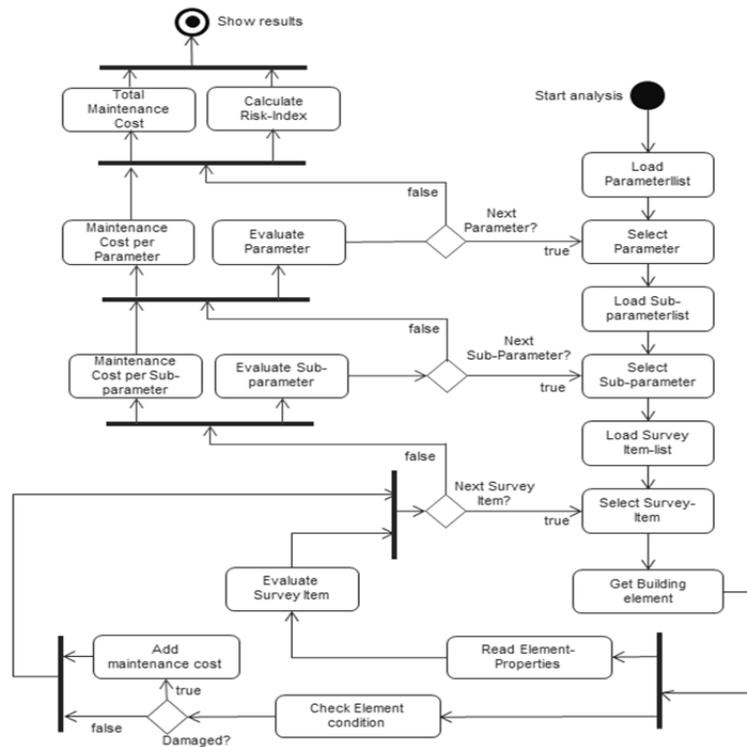
**Figure 3. Algorithm for the calculation of risk index and maintenance costs.**
