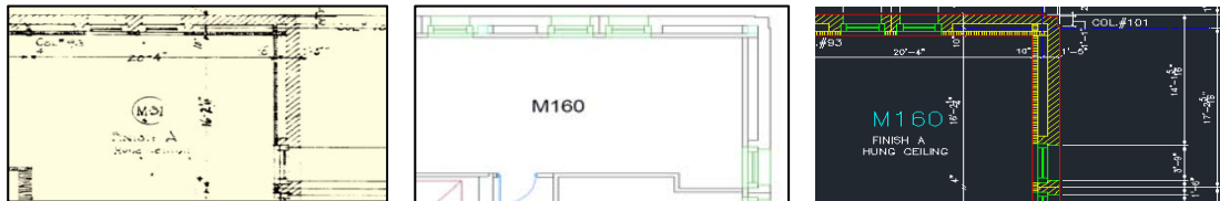
Figure 1. Difference among Various Formats: Scanned PDF, PDF and CAD
