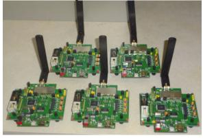
Figure 1. Nanotron swarm nodes (swarm of 5 nodes)
