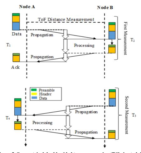
Figure 2. Symmetrical double-sided two way ranging (Röhrig et al. 2012)
