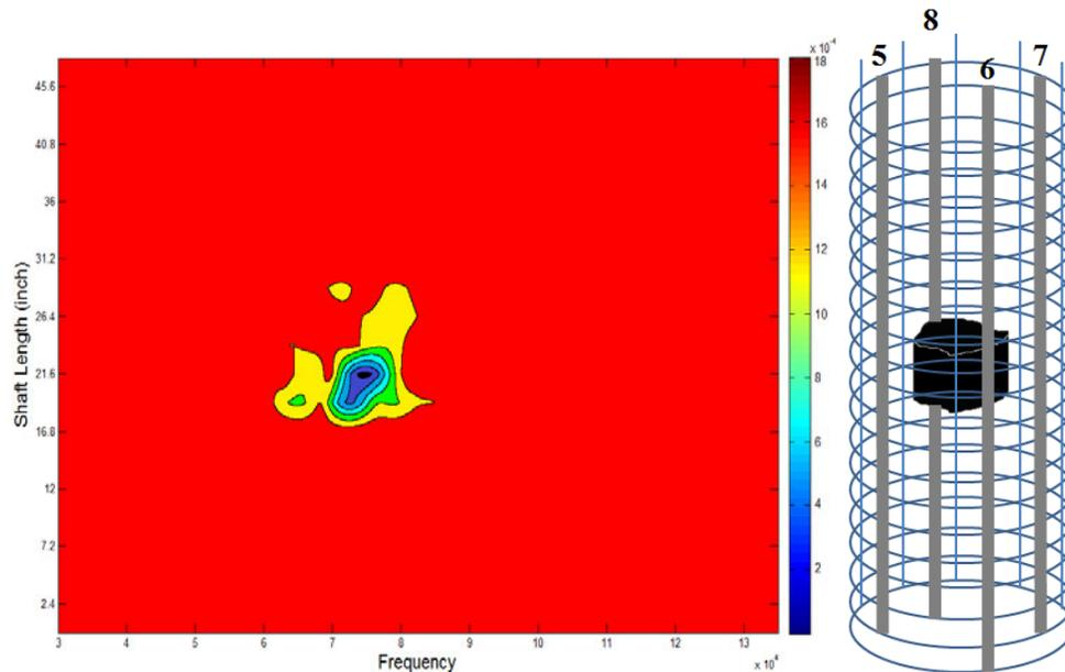
Figure 8. Frequency Domain Tomography (Specimen 2)
