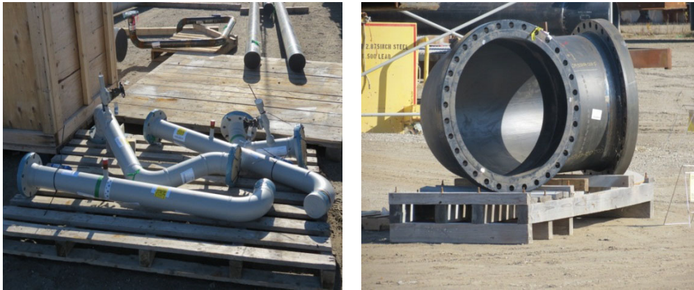
Figure 1. Prefabricated pipe spools to be shipped to construction sites. (Photos are taken by the author at an Aecon fabrication shop, Cambridge, Canada)
