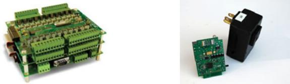
**Figure 2. Data Acquisition Hardware (a) Enersure (Source: Trendpoint Website 2013), and (b) Firefly(WiSE Lab Website 2013)**
