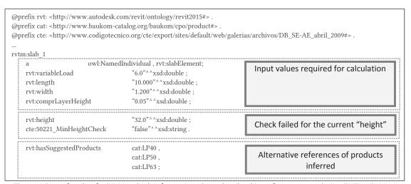
**Figure 8** Part of code of a BIM in which information about the checking of precast regulation EHE08:50221 is provided, and possible three valid product alternatives of the catalogue for an instance (rvtm:slab\_1) is suggested.
