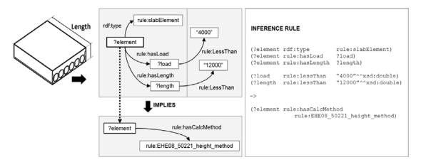
**Figure 4** Basic example of a rule (in JenaRule language) allowing to infer the most appropriate calculation method (namely, rule:EHE08\_50221\_height\_method) for elements of type rule:slabElement with a load less than 4000 KN/m² and a length less than 12000 millimetres.
