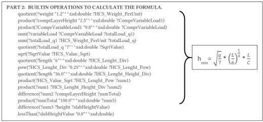
**Figure 6** Part of the rule describing the calculation according to the EHE 50.2.2.1 formula used to derive the minimum height of valid hollow-core slabs (PART 2).
