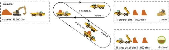
Figure 3: Set-up of the case study
