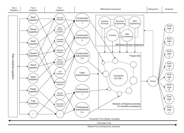
Figure 3 Conceptual view of typical BIM project CSC
