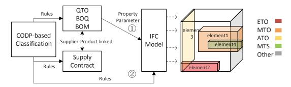
Figure 7 CODP-based supply information for IFC model
