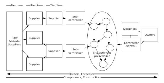
Figure 2 Conceptual view of the construction project supply chain
