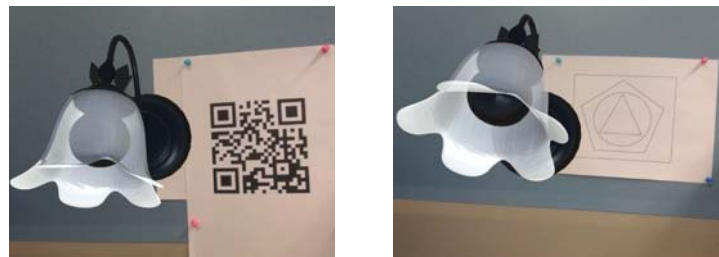
Figure 2. (Left) Result of marker-based AR using a QR code as the marker. (Right) Result of marker-based AR using simple geometries as the marker
