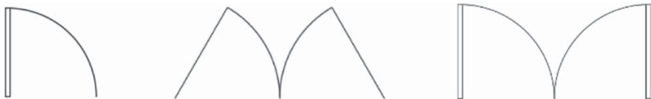
Fig. 9.5 Different shapes of door in real-life 2D drawings
