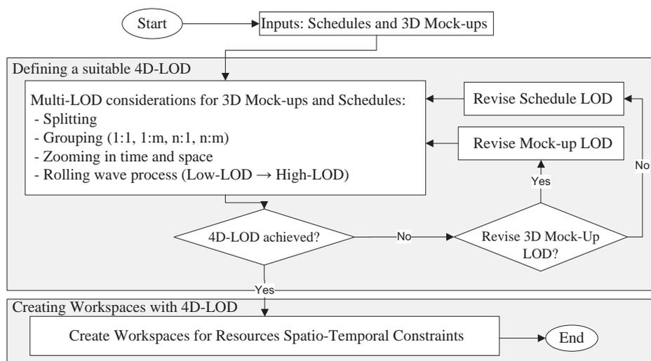
Fig. 10.1 Process of 4D-LOD adjustment
