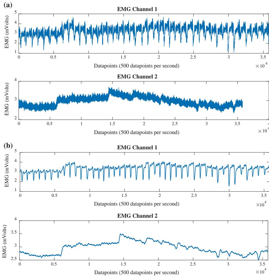
**Fig. 22.1** EMG signal artifacts removal: **a** Raw EMG signals recorded from a worker's bicep muscle (Channel 1) and shoulder muscle (Channel 2); **b** Filtered EMG signals
