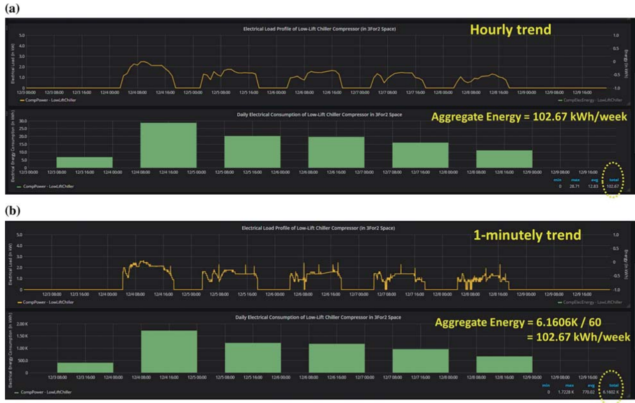
Fig. 77.3 Comparison of electrical power consumption profiles of a low-lift chiller compressor and its corresponding daily energy consumption represented as bar-charts for a week in Feb.'18 based on a 1-hourly trends b 1-minute trends
