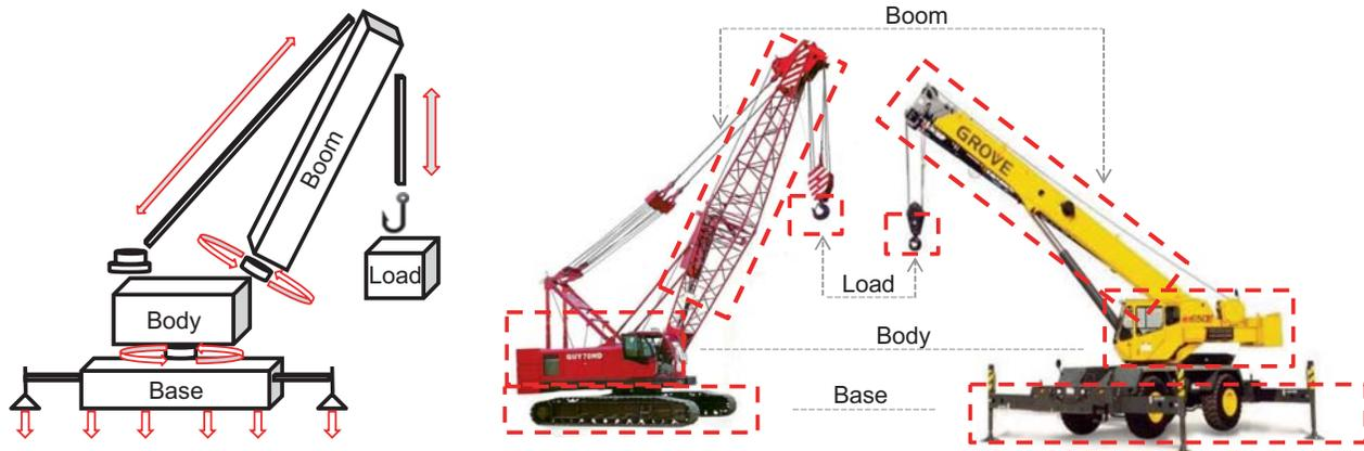
**Fig. 78.3** Representation of isolated crane modules
