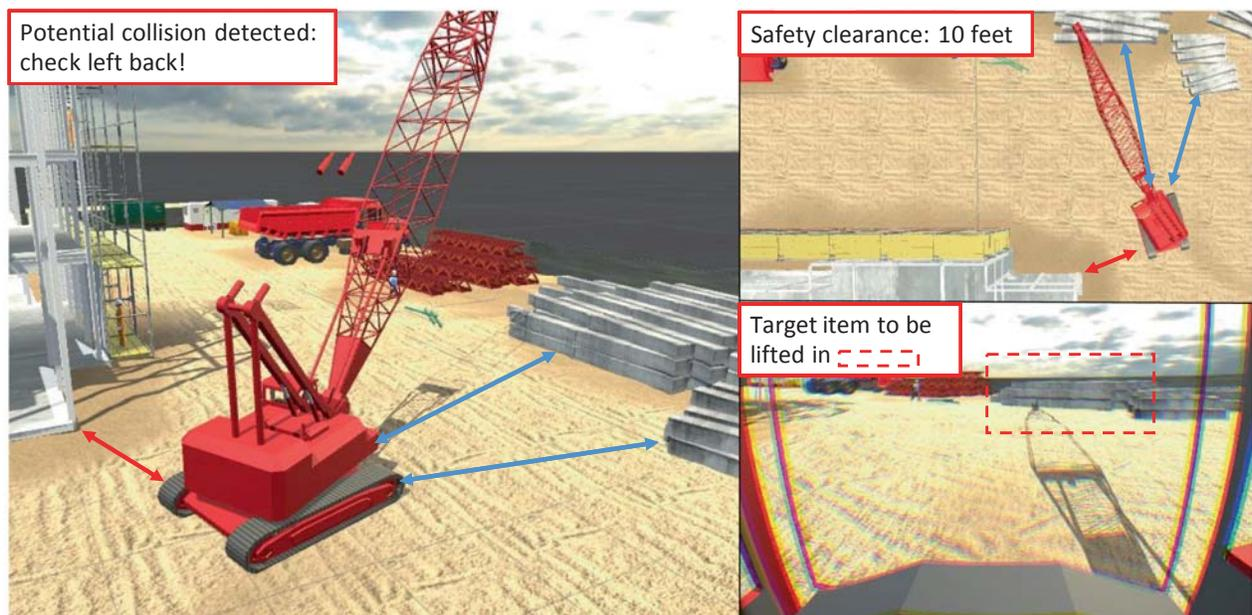
**Fig. 78.7** User interface: crane movement visualization [21]
