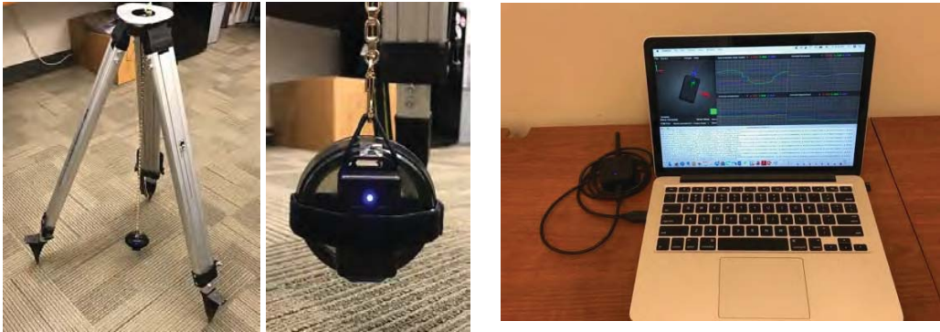
Figure 5: Load Sway Simulation: (a) tripod setup and (b) IMU sensor (left)
