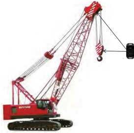
Figure 1: IMUs' Location on a Mobile Crane (left)
