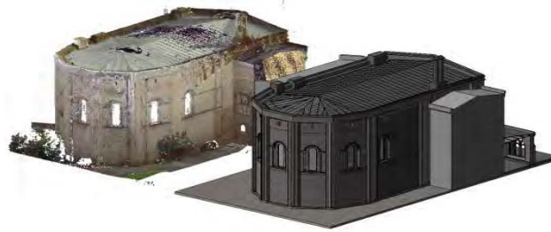
Figure 3: Point cloud data of Chapter House, Durham Cathedral and resulting BIM.
