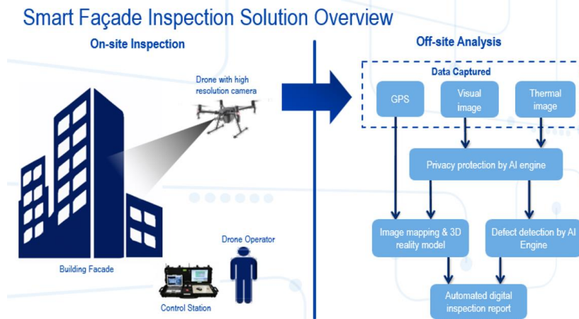
Figure 7. Smart Façade Inspection execution.
