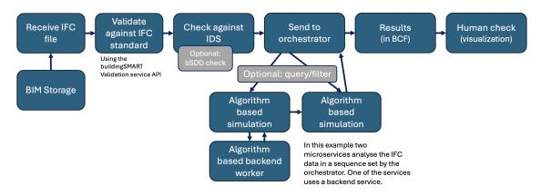
**Figure 1:** An example of different independent quality checking services combined using a service orchestrator to create one automated check process.
