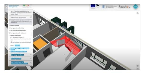
**Figure 2:** An example where the use of voxilisation showed that people can fall from the stair flight due to a lack of protection (railing, etc). Source: ACCORD demo country Estonia
