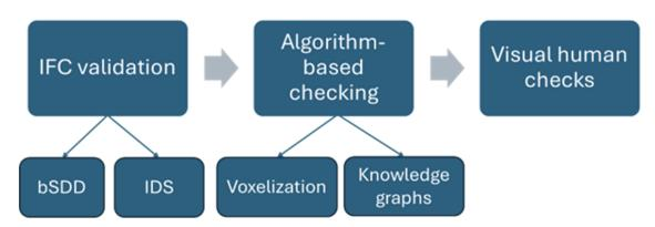
**Figure 4:** Steps (with suggested services and technologies) to improve the reliability of IFC files and compliance checks.
