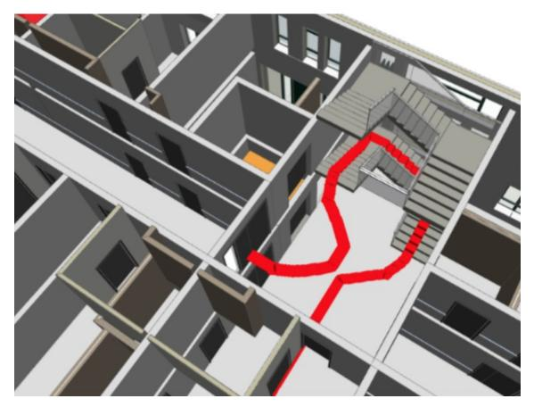
Figure 3: Visualisation of the calculated (derived) fire escape route.
