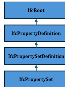
Figure 3. Entity inheritance of IfcPropertySet ( IfcObjectReferenceSelect - IFC 4.3.2 Documentation, 2022)
