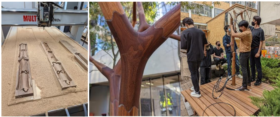
Figures 5,6, and 7 – Jig system on CNC bed, Nodal Connection Detail, Assembly Process of ECU
